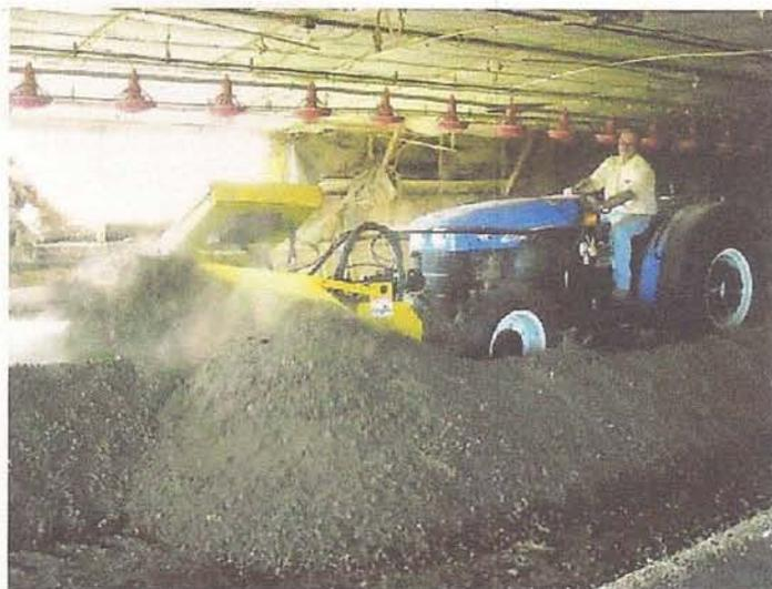
Figure 1. In-house composting of litter using Brown Bear aeration equipment.
